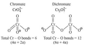
Total number of bonds between chromium and oxygen in both structures are 18.
